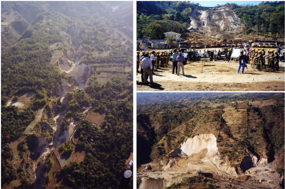
Photo.7 Geological and topographical condition in El Salvador is quite similar with Kagoshima. Surface ground is covered with very thick volcanic ashes so-called «tierra blanca». In this case, land failures in huge scale had been brought by the 2001 earthquake. But a heavy rainfalls also have the possibility to do the same thing next time.
