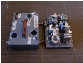
Photo.1 High-sensitive sensor with 3 components for microtremors.
